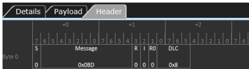
Figure 2(c). Drilling down to an even more detailed view of decoded data is shown here in bit/field boundary level decoding using a Keysight Infiniium S-Series oscilloscope.
